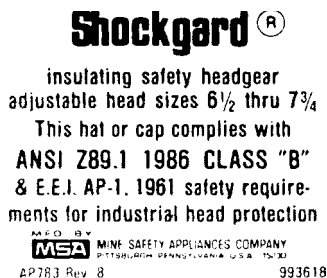
FIGURE 2.10 Hard hat label for a class E hard hat. (Courtesy Mine Safety Appliances Company.)
