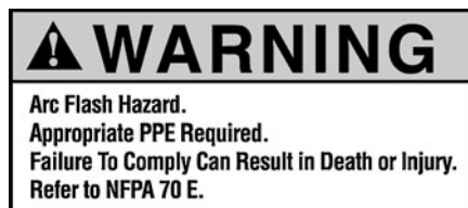
FIGURE 5.1 Minimum required warning label for posting on electrical equipment to warn of hazards.
