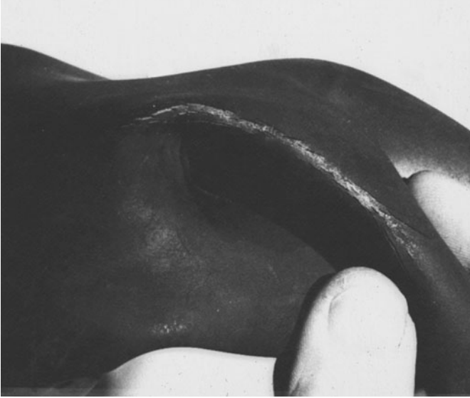
FIGURE 2.28 Age cracks. (Courtesy ASTM.)
