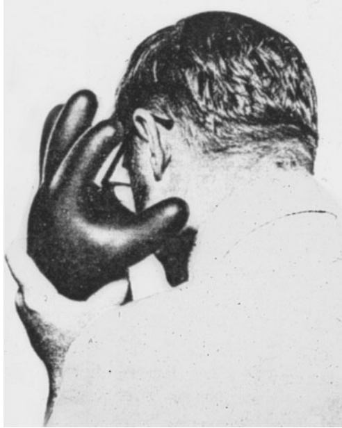
FIGURE 2.26 Inspecting rubber gloves by listening and feeling for air leaks through pinholes. (Courtesy ASTM.)
