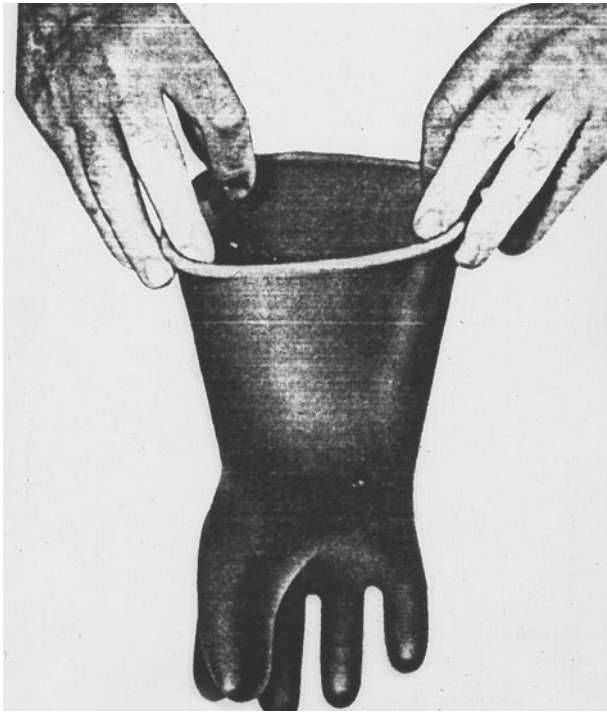
FIGURE 2.22 Inflating rubber gloves by twirling. (a) Grasping; (b) stretching; (c) twirling. (Courtesy ASTM.)
