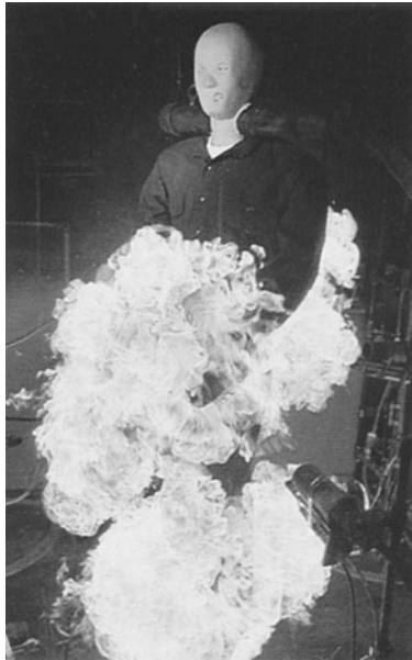
FIGURE 2.2 Thermal manikin used to generate the graph shown in Fig. 2.1. (Courtesy E.I. DuPont de Nemours.)
